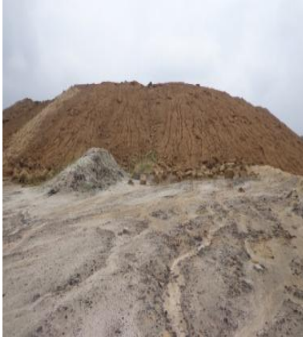
Plate -1: Top soil stacked on the inactive backfilled OB dump area
